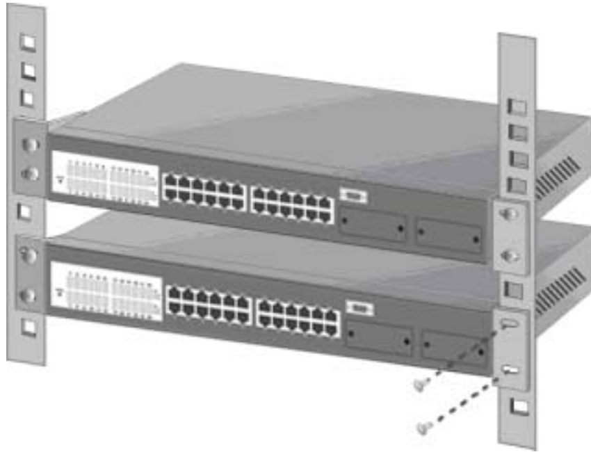
Figure 3-3. Mount the 24TP+1Fiber Module Switch in an EIA standard 19-inch Rack
